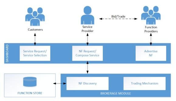
Figure 3-3 Brokerage module internal architecture
