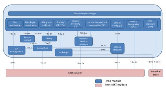
Figure 3-1 Brokerage module and its interfaces in the marketplace architecture
